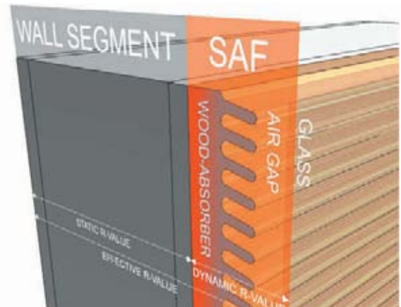
FIGURE 2: TYPICAL WALL SECTION WITH SAF ® . THE SAF ® SYSTEM WITH A WOOD ABSORBER, AN AIR GAP AND A PROTECTIVE GLASS COVER MOUNTED ON A MINIMALLY INSULATED STRUCTURAL WALL.
